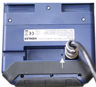
Fig. 69: Reset hole indicated by an arrow
