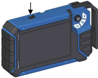
Fig. 16: Push button for pulling out the handle marked with arrow
