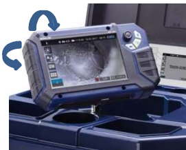
Fig. 12: You can turn and tilt the monitor
