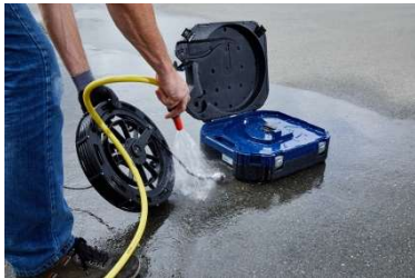
Fig. 77: Cleaning the viper and the rod
