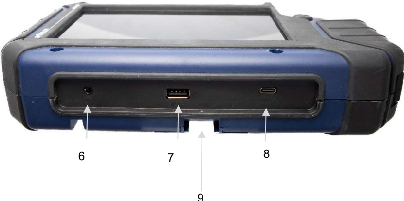
Fig. 8: Monitor bottom with connector strip
