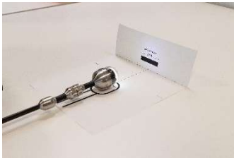
Fig. 49: Calibration with calibration template
