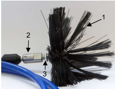
Fig. 4: Cleaning attachment (1) coupling with female thread M10 (2) and locknut (3)
