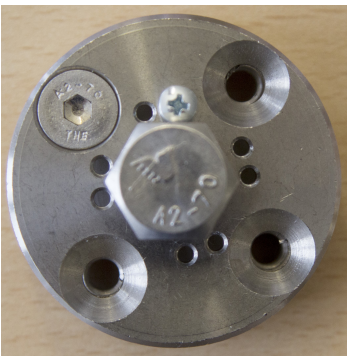
Fig. 8. End piece for holding chains with hexagon screw, secured by a security screw M3, 4 mm
