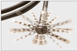
Fig. 5: Endpiece with chains driven by the drill
