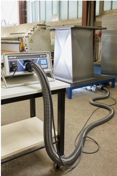
Fig. 12: Example: Measurement according to DIN EN 15727
