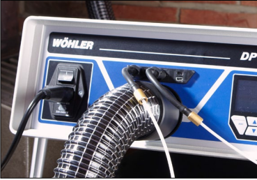
Fig. 37: Capillary hoses connected to the Wöhler DP 700 for the differential pressure measurement
