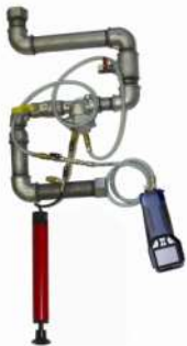
Fig. 55: Volume measurement with the Wöhler DC 410 FLOW and a syringe (up to 100 ml tube volume).
