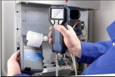
Fig. 60: Transmission of data records from the DC 410 FLOW to the thermal fast printer TD 600.
