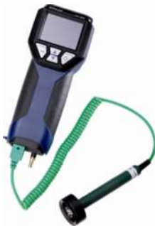
Fig. 5: Connecting the Special Wall Temperature Probe for measuring the heat transmission coefficient
